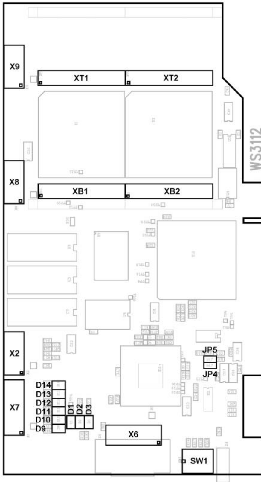
Picture 1: Top View of WS 3112 Board with Connectors, Jumpers, DIP-Switch
